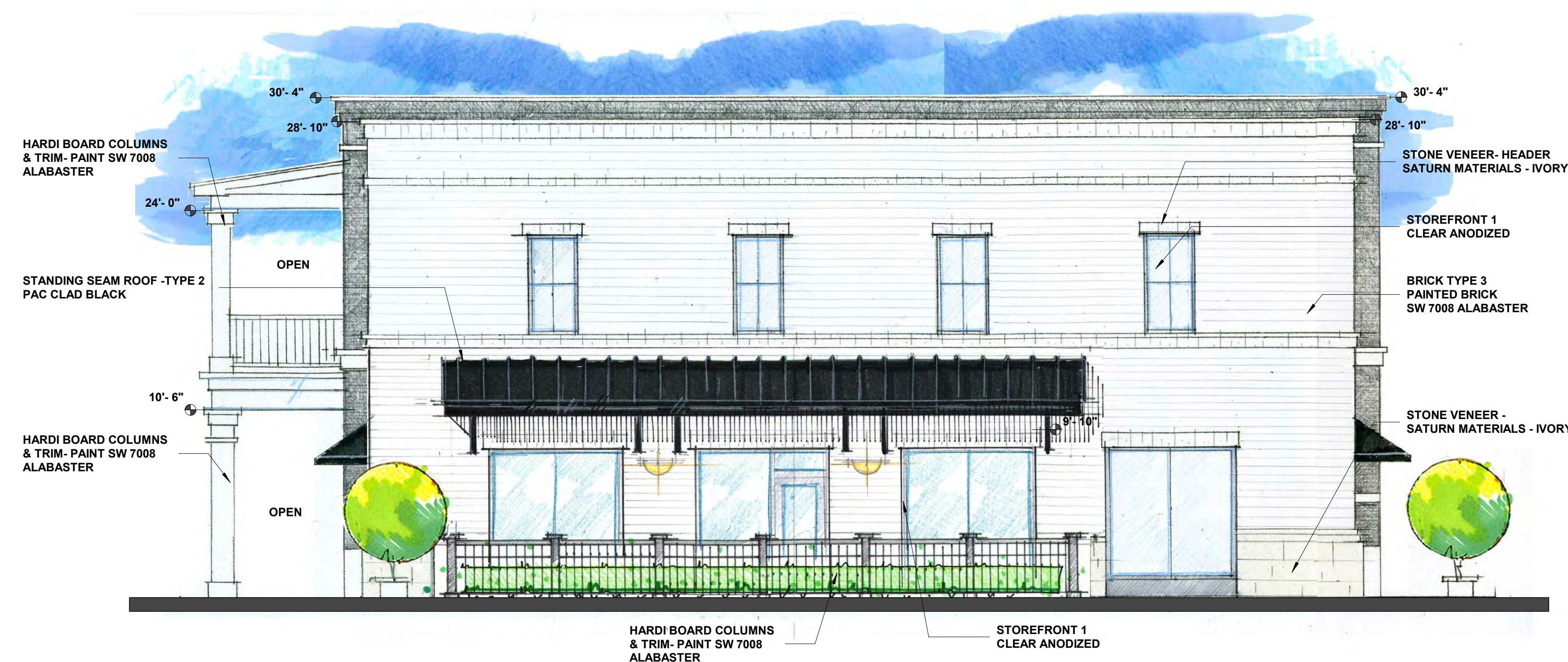
2 US 70 HIGHWAY ELEVATION - DRC 3/16" = 1'-0"
