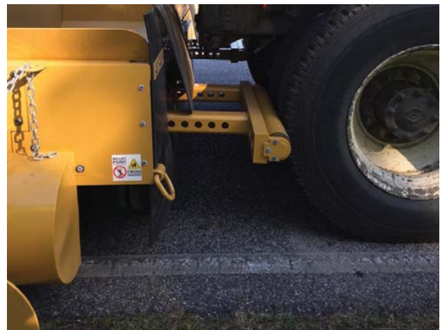
Rollers are adjustable to accommodate various truck axles.
