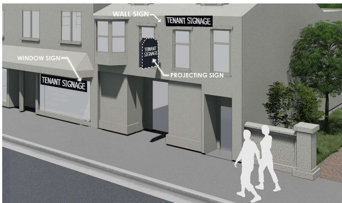
Figure III.5.6 Illustrative Example of Building Signs
